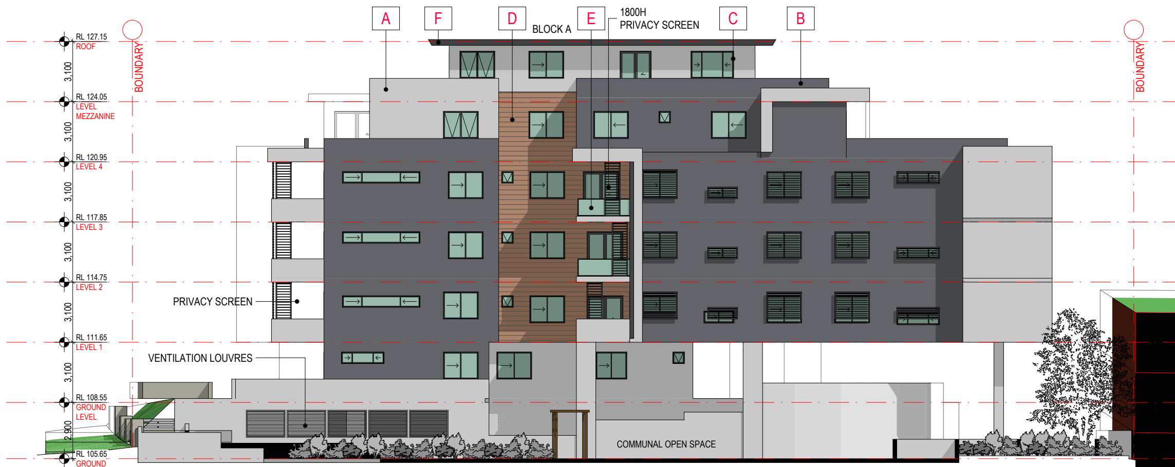
Elevation West - Block A 1:200
